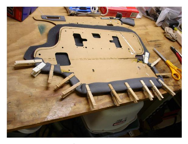
6. Fold over the edge and fasten it with cloths pins until dry.
