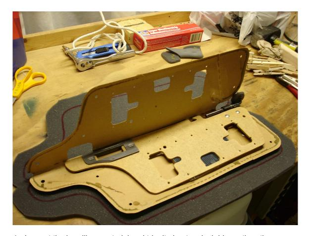
4. Lay out the headliner material and trim it about an inch bigger than the carboard.
