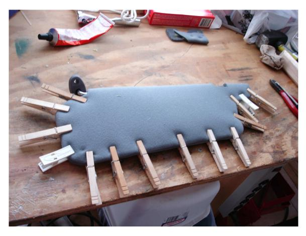
8. Apply glue around the edge, insert the mounting hardware and fold over the sun visor. Again fasten with cloths pins to hold until dry.
