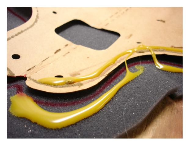
5. Follow your glue directions and apply the glue on the cardboard and on the headliner (foam side) so that when you fold the fabric over onto the cardboard, the glue will touch. Let it sit according to the directions.
